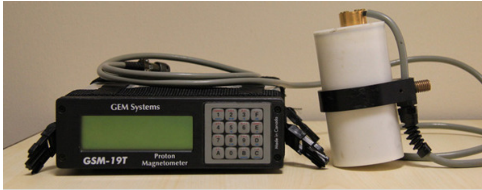
Figure 11: GEM GSM-19T proton precession magnetometer.
