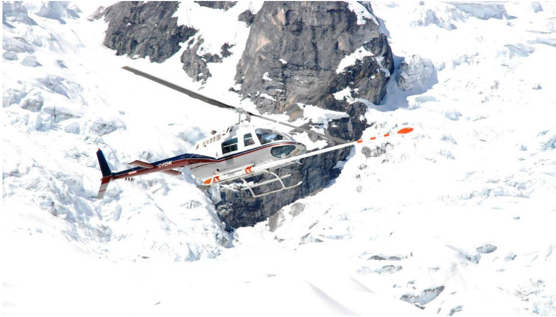
Figure 7: Bell 206 Jet Ranger equipped with mag stinger for magnetic data acquisition.
