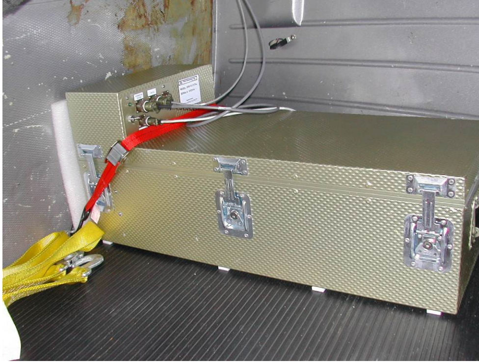
Figure 10: IRIS strapped into the cargo box of the helicopter.
