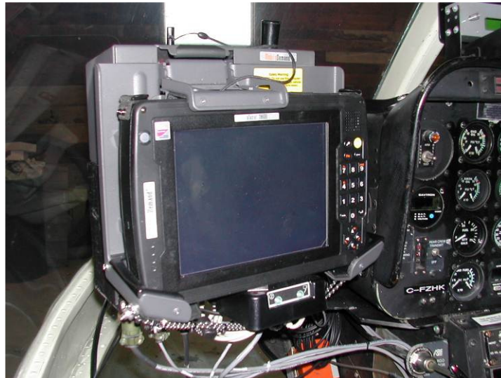
Figure 8: AGIS installed in the Bell 206.
